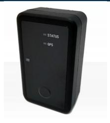
Rugged, waterproof, cellular GPS tracking device designed for tracking non-powered, exposed assets where super-long battery life is essential. The device works on 4G Cat-M1 networks. It comes in 2 options with Replaceable or Rechargeable battery. The replaceable option can last 7 years sending one event a day. Rechargeable option can last 1 year.
